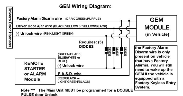
If the vehicle DOES NOT have a Factory Alarm OR Factory Keyless Entry, the GEM Wire Diagram is not used and you then wire the Door Locks up as a TYPE "C" Door Lock System.
