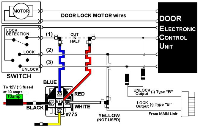
\* it has been noted that on the 2003 IS300 that if the doors will lock and unlock when the door is opend but when the door is closed the unit will lock but not unlock attach pin 87 or the YELLOW wire from the relay to Ground.
