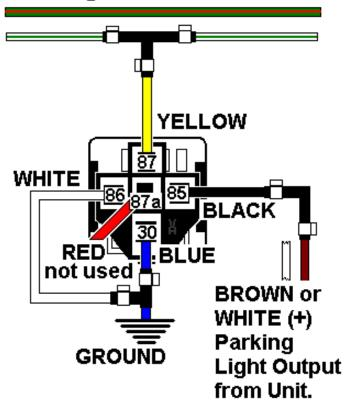
If your Unit has a (-) Negative Parking Light Output you can Connect directly without a Relay.
