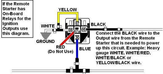
Connect the BLUE wire (Pin #30) to the (-)Negative Ignition wire that is comming from the Ignition Switch and is heading towards the Relay in the vehicle.
